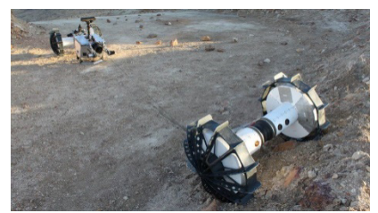
Tethered rover to explore lunar pits
