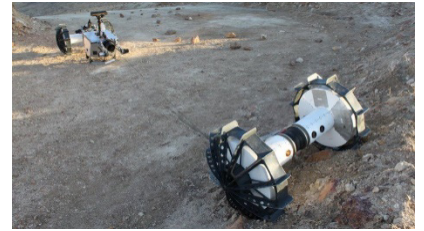
Tethered rover to explore lunar pits
